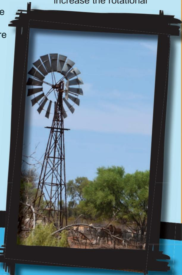
converted to the plunger motion by means of a crank. One turn of the wheel converts to one complete up-and-down stroke. Direct acting mills allow for deep bores which need slower pumping and more torque, as against low lift situations where geared windmills are most efficient.
